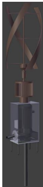
Figure 25: The final design of the pumping system along with wind turbine and internal component placement.
